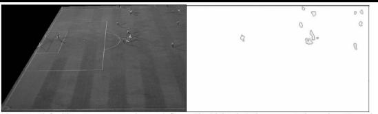
Figure 1: (left side): One camera view and figure 1b: (right size) the segmentation using: 1) motion filtering and 2) players' segmentation.
