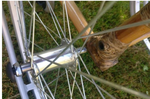
Close-up view of the joints of the bamboo wheelchair
