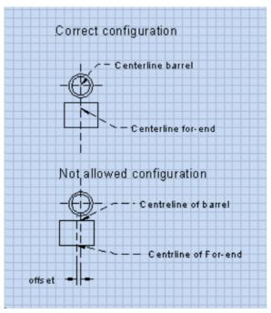
5.2 One side of the for-end must touch one side of the yoke.
