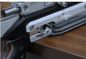
Trigger adaptation: trigger is outside the trigger guard and outside the dimensions of ISSF Rules.
