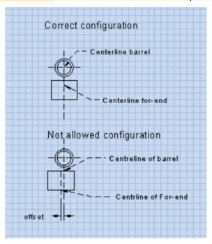
One side of the for-end must touch one side of the yoke.
