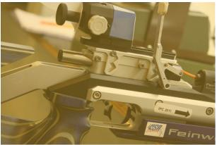
**Trigger extension:** trigger is inside the dimensions of ISSF Rules and protected by a trigger quard.
