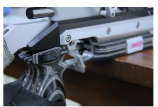
**Trigger extension:** trigger is inside the dimensions of ISSF Rules and protected by a trigger guard.
